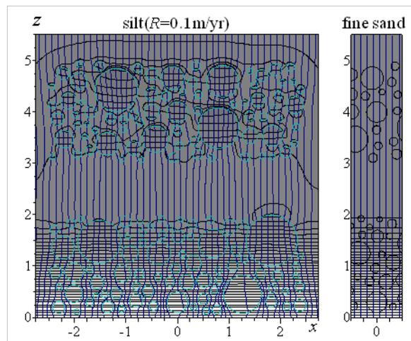
Vadose zone pressure head for silt embedded within fine sand (manuscript in preparation)
