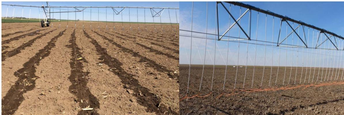
Figure 1. The Mobile Drip Irrigation technology (MDI) featuring the drip hoses on a center pivot irrigation system. Photos from [www.dragonline.net](http://www.dragonline.net).
